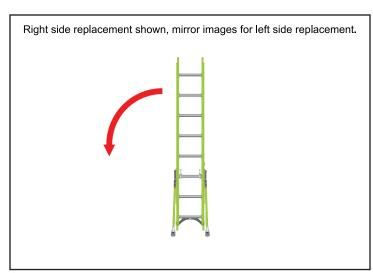
2. Lay the ladder on its side with the outrigger being replaced facing up.
