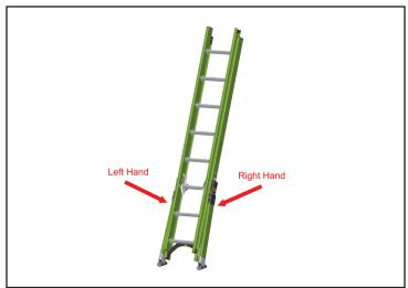
1. Identify the outrigger being replaced. Confirm the foot on this outrigger faces the same direction as the one in the kit. If it does not match, please call our Customer Experience Team at 800-453-1192 for assistance.
