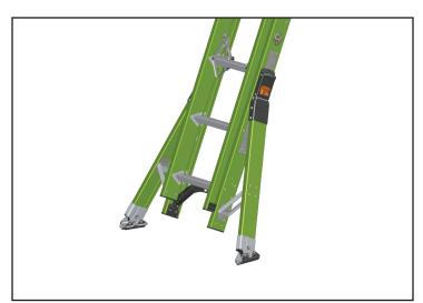
11. Confirm new outrigger is secure and functioning properly before use.
