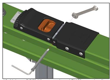
10. Using a 5/32" Allen wrench and 7/16" wrench, align and tighten the new shoulder bolt and lock nut.
