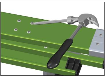
4. Use a hammer and chisel to remove any excess rivet head material from the rail.
