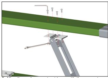
8. Align the replacement outrigger with the support arm bracket. Using a 1/8" Allen wrench and 3/8" wrench, tighten the new socket cap screws and lock nuts.
