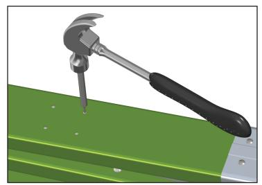
5. Use a hammer and punch to completely remove the drilled rivets.
