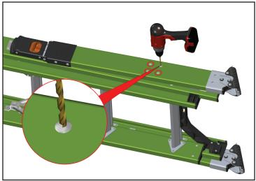
3. Using a 3/16" drill bit, drill through the rivet heads connecting the outrigger to the support arm.
