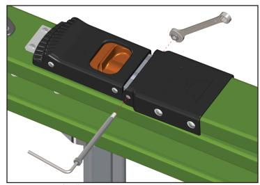
6. Using a 5/32" Allen wrench and 7/16" wrench, remove and discard the existing shoulder bolt and lock nut.
